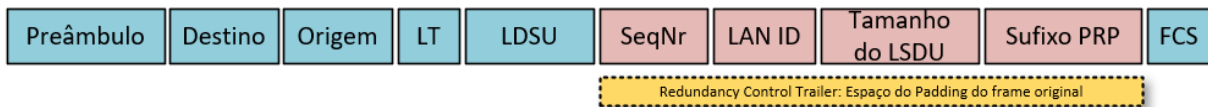
FIGURA 4 – O Redundancy Control Trailer do LRE usando o campo Padding do frame Ethernet original
